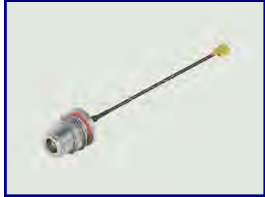
P/N:20050913-01 Con1: N(F) S/T Bulkhead Jack With O-Ring Cable: 1.37mm Con2: IPEX (2.5H)
