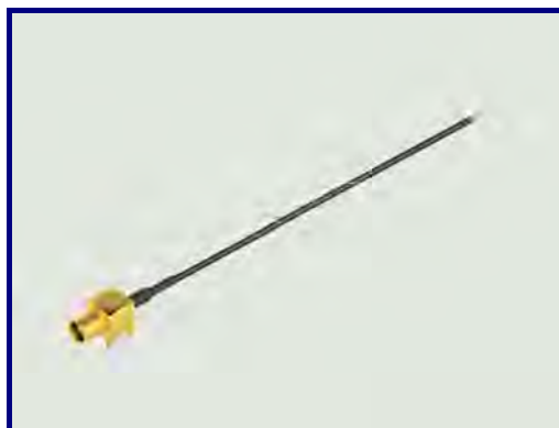
P/N:20081216-02 Con1: MCX(F) R/A Jack For P.C.B Mount Cable: 1.32mm Con2: Strip&Tin
