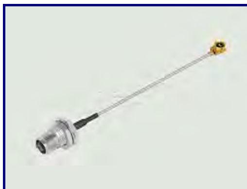
P/N:20070730-02 Con1: TNC(F) S/T Bulkhead Jack Cable: 1.32mm Con2: IPEX (2.5H)
