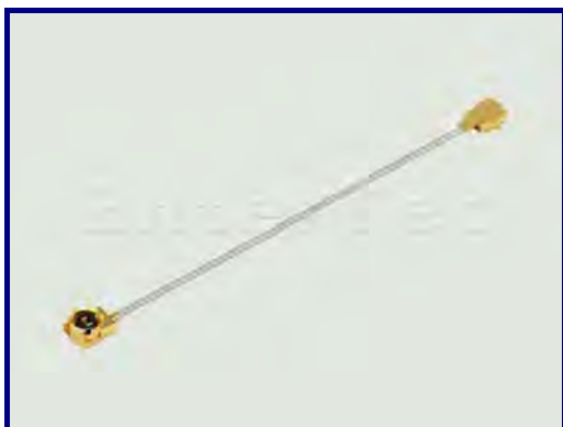
P/N:20061220-02 Con1: IPEX (2.5H) Cable: 1.32mm Con2: IPEX (2.5H)
