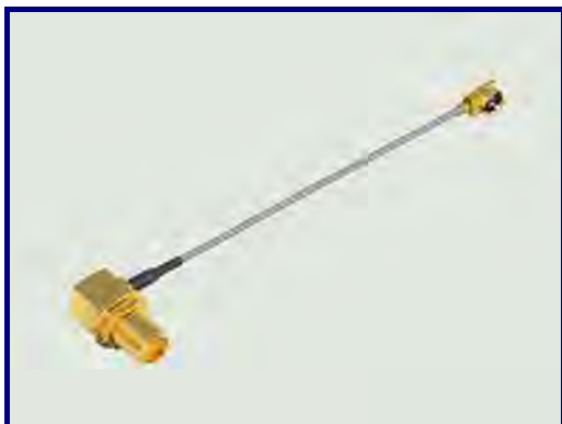
P/N:20060413-01 Con1: SMA(F) R/A Jack Cable: 1.32mm Con2: IPEX (2.5H)
