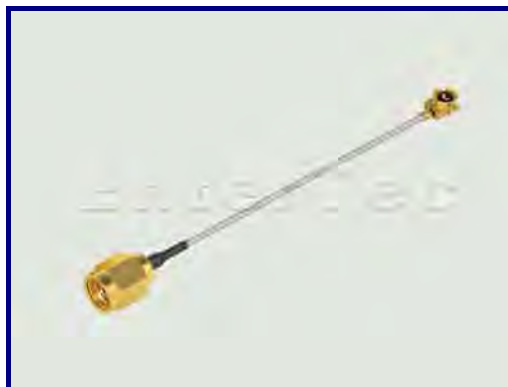
P/N:20061108-01 Con1: SMA(M) S/T Plug Cable: 1.32mm Con2: IPEX (2.5H)
