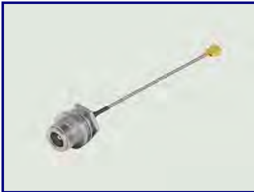
P/N:20070607-08 Con1: N(F) S/T Bulkhead Jack Front Mount Cable: 1.37mm Con2: IPEX (2.5H)
