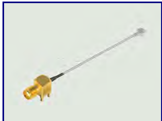
P/N:20080813-02 Con1: SMA(F) R/A Jack And P.C.B Mount Cable: 0.81mm Con2: Murata MXTK92
