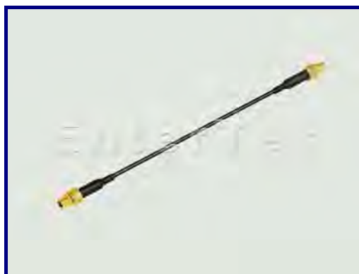
P/N:20080114-04 Con1: MMCX(M) S/T Plug Cable: 1.32mm Con2: MMCX(M) S/T Plug
