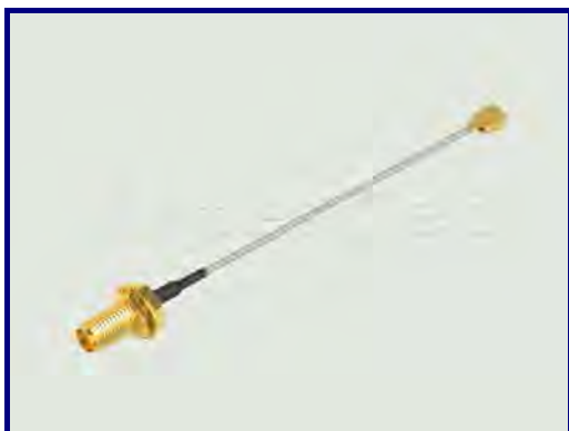
P/N:20070730-04 Con1: SMA(F) S/T Bulkhead Jack Cable: 1.32mm Con2: IPEX (2.5H)
