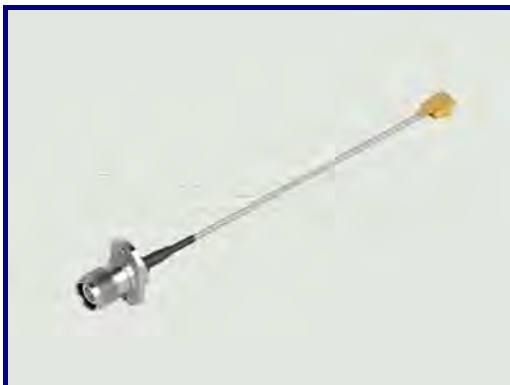
P/N:20080407-02 Con1: TNC(F) S/T R/P Jack Cable: 1.37mm Con2: IPEX (2.5H)
