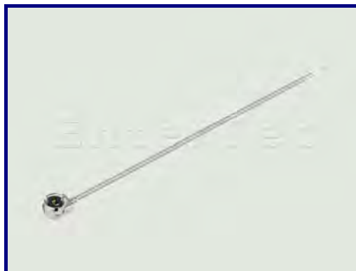
P/N:20061012-01 Con1: U.FL (2.5H) Cable: 1.32mm Con2: Strip & Tin
