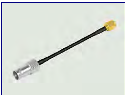
P/N:20060713-01 Con1: BNC(F) S/T Jack Cable: RG-174 Con2: SMA(M) S/T Plug
