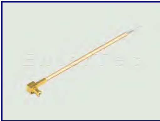
P/N:20080416-04 Con1: MCX(M) R/A Plug Cable: RG-316 Con2: Strip & Tin
