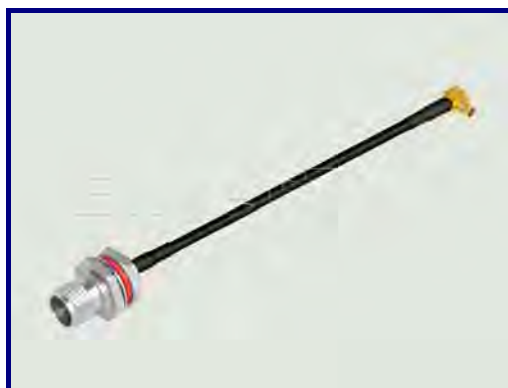
P/N:20061127-01 Con1: TNC(F) S/T Bulkhead Jack Cable: RG-174 Con2: MMCX(M) R/A Plug
