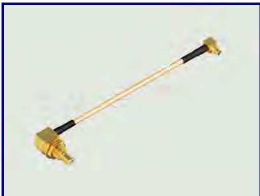
P/N:20060926-02 Con1: SMB(M Contact) R/A Bulkhead Jack Cable: RG-178 Con2: MMCX(M) R/A Plug
