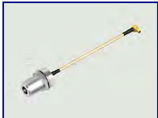
P/N:20071212-01 Con1: N(F) S/T Bulkhead Jack Cable: RG-316 Con2: MCX(M) R/A Plug
