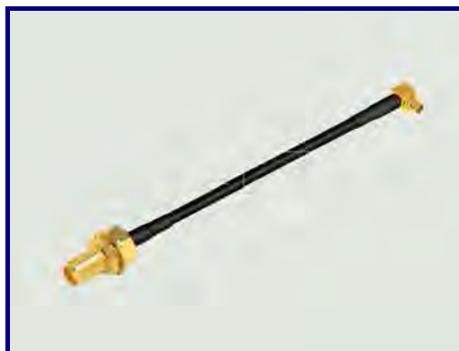
P/N:20080419-02 Con1: SMA(F) S/T Bulkhead Jack Cable: RG-174 Con2: MMCX(M) R/A Plug
