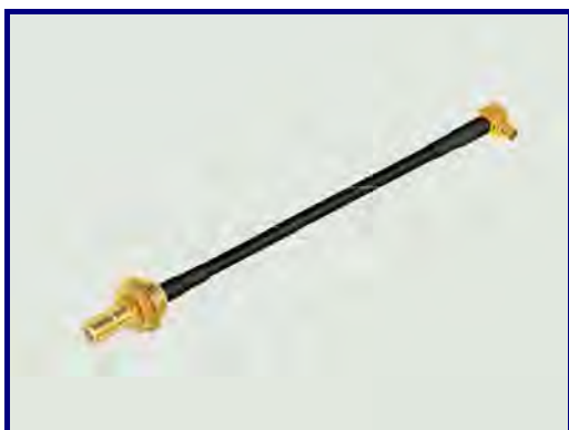
P/N:20071213-02 Con1: SMB(M Contact) S/T Bulkhead Jack Cable: RG-174 Con2: MMCX(M) R/A Plug
