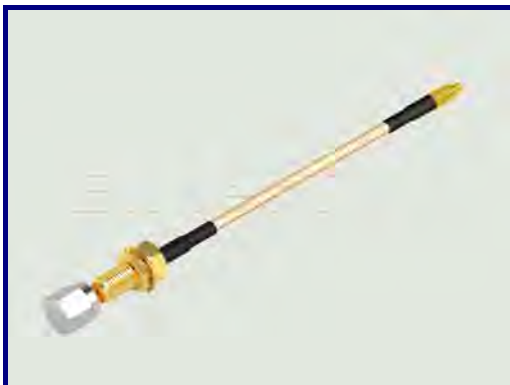
P/N:20080218-01 Con1: SMA(F) S/T Bulkhead Jack + Protective Cap Cable: RG-316 Con2: MMCX(M) S/T Plug
