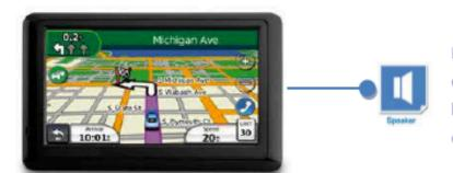
It is used to emit a signal sound or navigation directive when button is pressed or navigation directive is shown.
