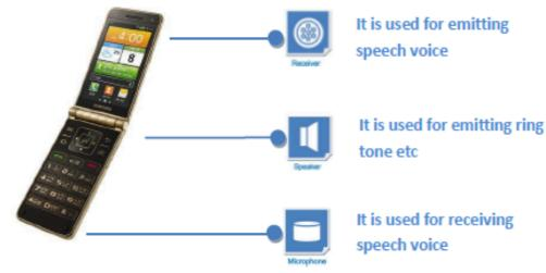
The flip or clamshell is a mobile phone form factor which is in two or more sections that fold via a hinge. If the hinge is on a long edge the device is more likely to be called clamshell than flip phone (e.g., Nokia Communicators).
